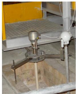
Examples of installed HOLDING and MOUNTING DEVICES
